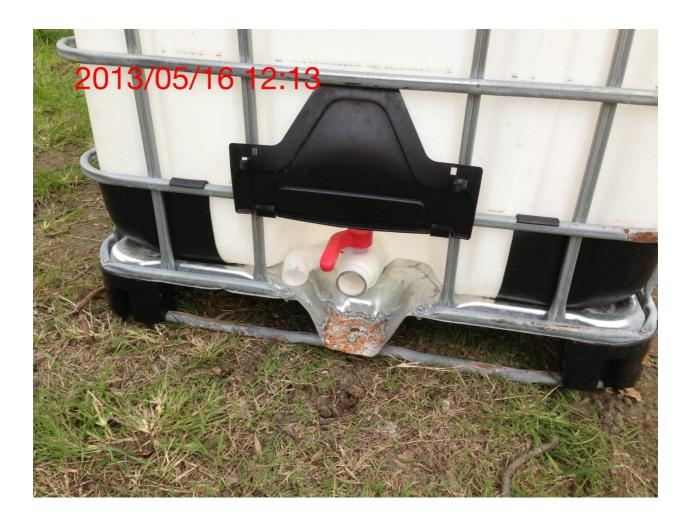
Photo of the open IBC tap, and the spilled chemical on the ground where the reaction took place.  $\label{eq:continuous}$
